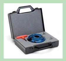
The set consists of a 132 mm diameter head with two r=15ad r=20 mm knives mounted on the tool and two spare r=12 and r=18 mm knives. Head is manufactured in light alloy.
