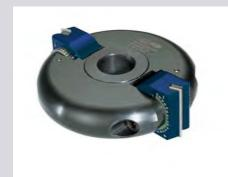
Cutterhead with HW reversible knives. The two wings are adjustable degree by degree from 0° to 70°. Due to the particular construction, this tool is of universal use. The tool can also be used as a rebate cutterhead if matched with element B (spur holder) and if wings are positioned at 0°.
