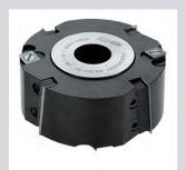
Cutterhead with two alternate shear knives and light alloy body for extremely accurate rebates. Suitable for solid softwood, chipboard, veneered and laminatedd panels, plywood, etc.
