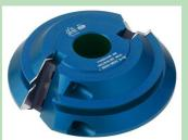
Cutterhead in light alloy with two knives for  $45^{\circ}$  joints. The joint is obtained by two subsequent working phases: the first with the piece being worked in horizontal position and the second with the piece of wood in vertical position.
